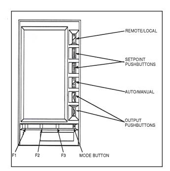
Figure 2: MC5000 Operator Keys
